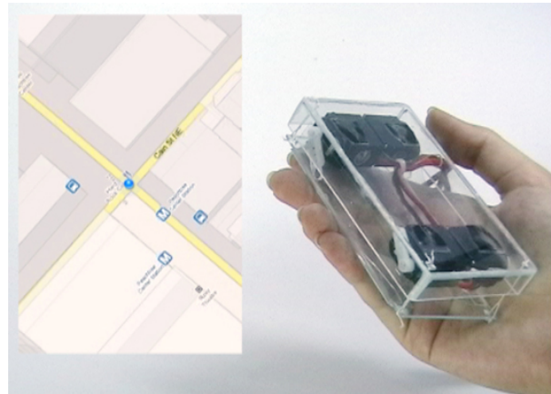
FIGURE 5.11: The Shape-Changing Mobile (two-dimensional version). Application: »haptic compass«. The device provides directional information by thickening towards the destination's direction while navigating.
