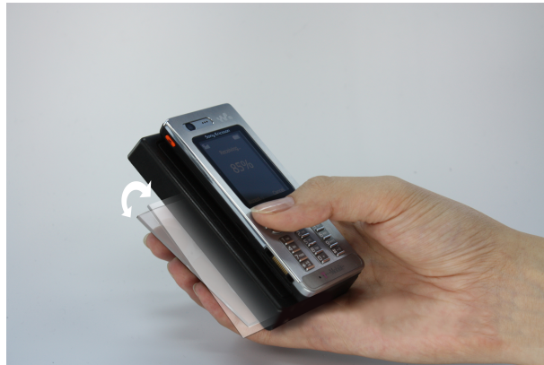
FIGURE 5.2: The Shape-Changing Mobile (one-dimensional version).
