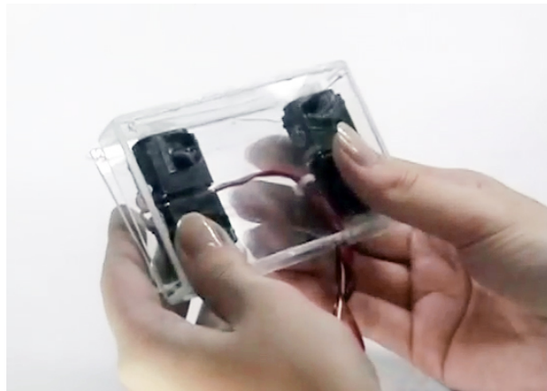
FIGURE 5.9: The Shape-Changing Mobile (two-dimensional version). Application: »actuated ergonomics«. The device can be thin in the pocket, and dynamically adjust its shape when held in hands.
