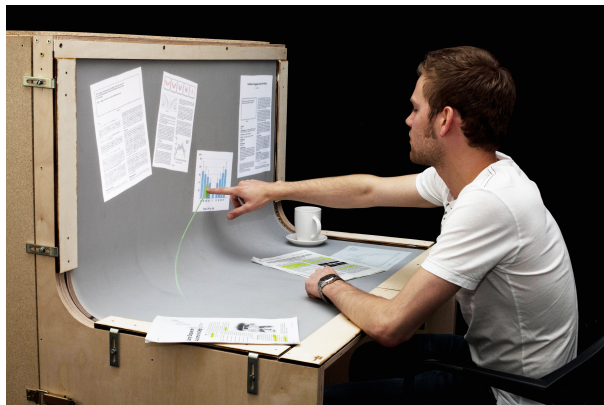
FIGURE 2.3: »BendDesk« by Weiss et al. (2010) integrates multi-touch interaction into a curved desk.
