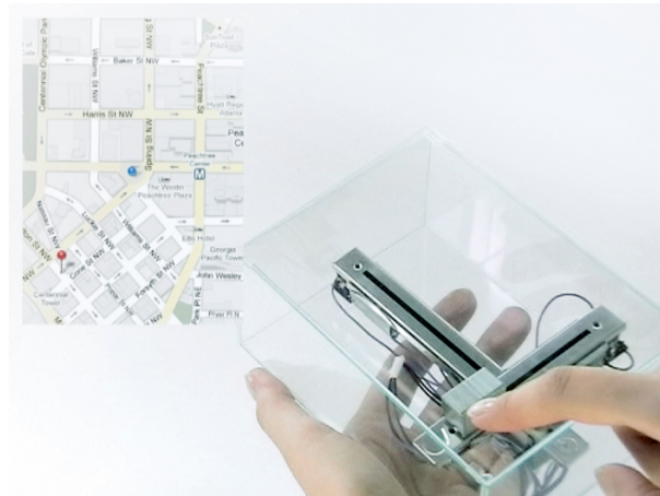
FIGURE 5.25: The Weight-Shifting Mobile (two-dimensional version). Application: »GUI augmentation«. Digital contents are displayed visually and through the device's centre of gravity.
