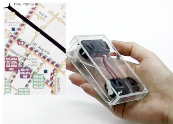
FIGURE 5.10: The Shape-Changing Mobile (two-dimensional version). Application: »augmenting GUI contents with thickness«. The device displays off-screen content through thickening towards the location of the content.
