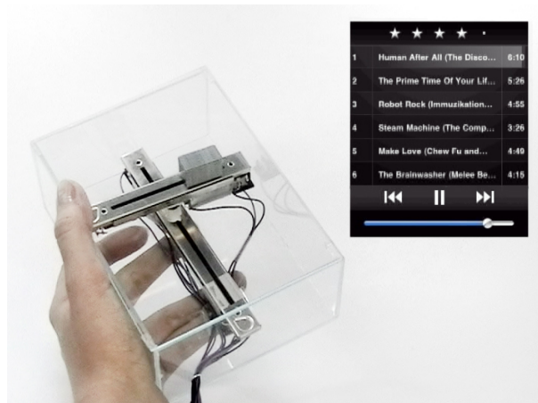
FIGURE 5.26: The Weight-Shifting Mobile (two-dimensional version). Application: »ambient display«. A music player's playhead position and playlist progress are displayed by the device's centre of gravity.
