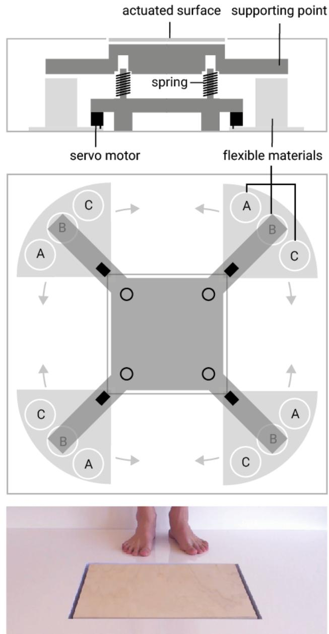
Figure 4. The supporting points of the upper frame can be set to different materials and therefore users can explore three degrees of rigidity
