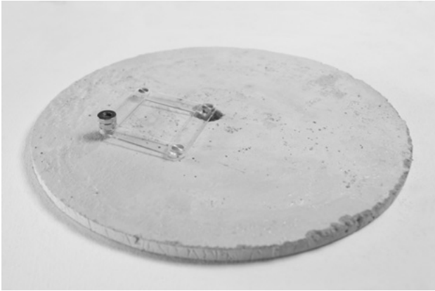
Figure 4: Concrete Data: a stone-based data logger.
