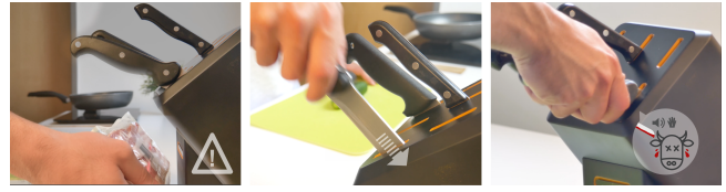
Figure 3: The ‘Cut’: a knife block that requires users to scan products before letting them cut, and – through a haptic feedback mechanism – requires them to brutally stab the knife back after cutting meat, causing a feeling similar to kill an animal.
