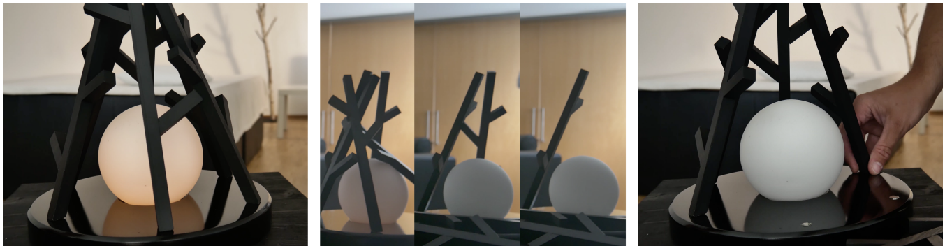
Figure 1: The ‘Fireplace’: a lamp that uses electromagnetically fixed logs to symbolize kilowatt hours used in the household and drops the logs over the course of a day, requiring users to carefully put the logs back, in order to restore electricity.
