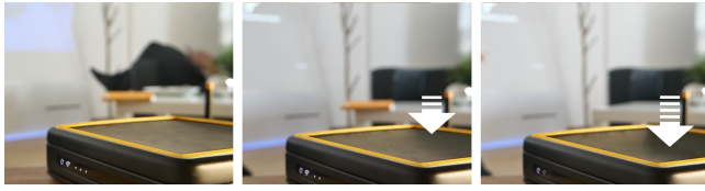
Figure 2: The ‘Router’: a shape-changing wireless access point which physically runs empty as data is used over the day (and, thus, attention diminishes). It also requires users to calmly touch it to restore connectivity, forcing them to pause and contemplate for a moment.
